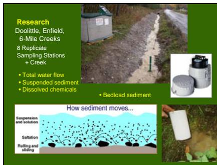
In-depth monitoring is quantifying the amounts of water, suspended sediment, dissolved chemicals, and bedload sediment that ditches are contributing to Doolittle Creek, near Candor, NY. Bedload pitfall traps capture the pebbles and gravel that are too heavy to move suspended in the water, but instead bounce and roll along the bottom.
